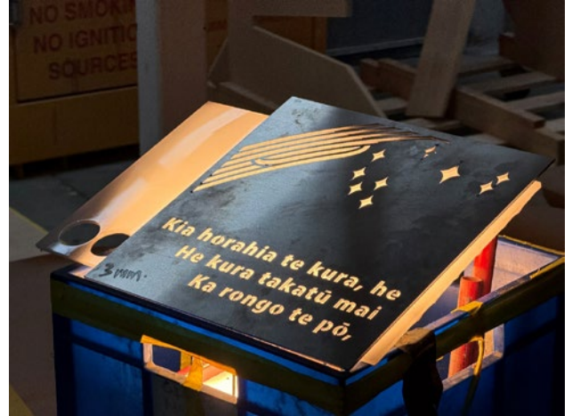
Testing laser-cut text and design elements into aluminium for the sculpture. Design: David Hakaraia. Manufacture: Human Dynamo Workshop. Credit: Human Dynamo Workshop.
